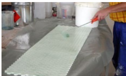
Hand lay-up laminate
