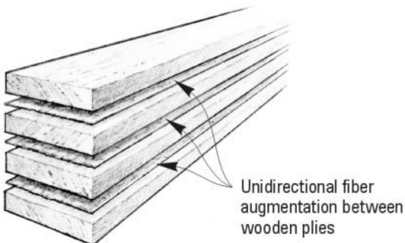
Because wood has a number of natural flaws, it is wise to take precautions to reduce or diffuse them with a grading procedure. After a board has been ripped into thinner plies, flip alternate pieces end-
