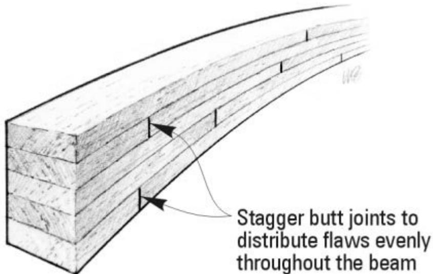
Often it makes sense to place high-modulus/high-strength wooden plies, such as ash or mahogany, furthest from the neutral axis (top and bottom), and lighter, weaker materials such as cedar or spruce in the center. This method puts the stronger, heavier materials where the loads are the greatest and lighter materials where the loads are less, much like building an I-beam. It offers greater strength with less weight.
