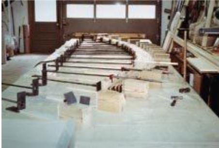
The beams were tapered in profile, and it is tough to taper a laminate with saws and planes. We suggested that they taper the individual laminate layers before laminating. That way, after gluing the layers together, only the sides of the beams would need to be planed. The resulting beams with their tapered layers would also be more aesthetically pleasing. In addition, less end grain would be exposed than if the top or bottom of the beam were sawed to shape after lay-up.
