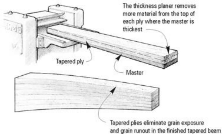
A good way to beef up a unidirectional wood laminate is to augment plies with unidirectional synthetic reinforcing fibers-fiberglass, carbon, Kevlar-adding considerable strength with a minimum weight gain. Strength can be improved further by placing these materials away from the neutral axis of the beam.
