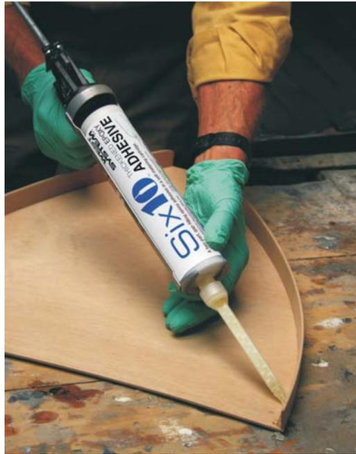
With the 600 Static Mixer attached to the Six10 cartridge, it's easy to lay down a bead of thickened epoxy adhesive right where you need it.
