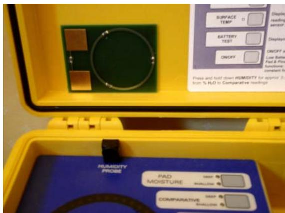
1. Ensure the lid is in the upright position and there is nothing behind the calibration check unit -including fingers!
