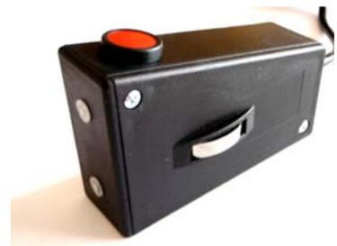
LED displays the temperature difference. Where the substrate temperature is lower, then as the thermistor readings approach dew point the coloured LED traffic lights will illuminate, going from green, to amber and finally to red, indicating the substrate is **below dew point**.
