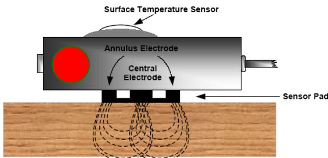
The substrate is penetrated by the electric field emanating from an electrode coupled to a stable low frequency oscillator.
